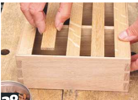
28 Thickness slats to 24 x 5mm and saw to length. These can be pinned or screwed into rebates
